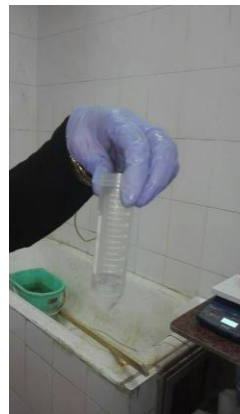
0.8 g NaOH in 10 mL ethanol (0.5% catalyst & 10% alcohol of the oil mass)
