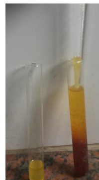
Separating the oil (upper layer) from the glycerol (lower layer)
