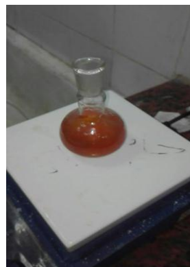
Heating the oil at 130 °C
