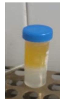
Adding some water to wash the oil from any residue, keep it two hours for separation
