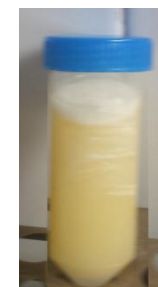
Adding some water to wash the oil from any residue, keep it two hours for separation
