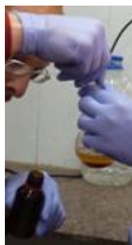
Separating the oil (upper layer) from the glycerol (lower layer)
