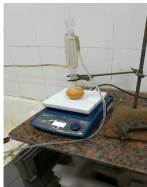
After stirring, keep it for 12 hours till cooling and the glycerol settle down
